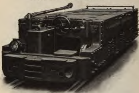
Side Frames of Box Construction
